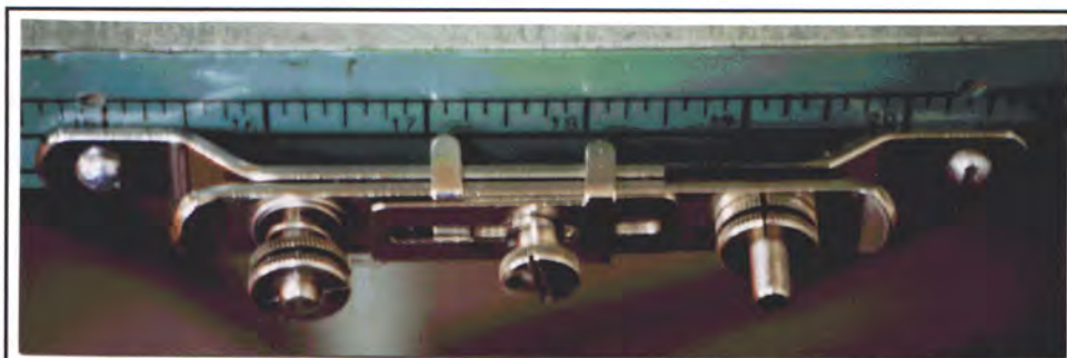
Figure 7: The elastic tensioning device which can be mounted on the sewing machine table to tension and guide the tape .
