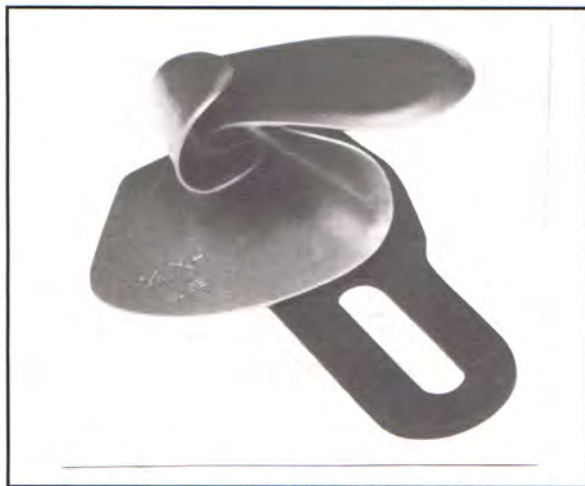
Figure 1. A Seam Folder which mounts in front of the presser foot on a sewing machine.
