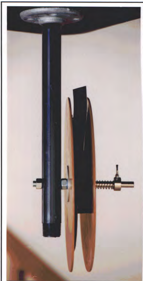
Figure 5: The reel, with its pipe flange base and plastic pipe column.
