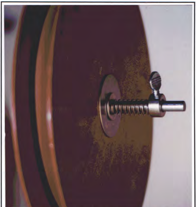
Figure 6: The end of the reel axle showing the reel tension assembly components.
